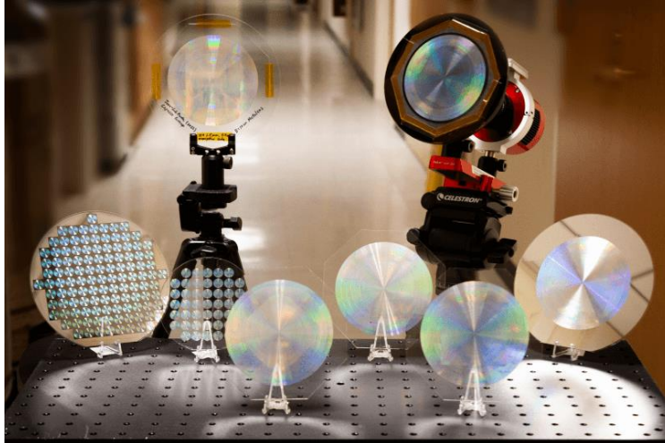
This 10-centimeter-diameter glass metalens can image the sun, the moon and distant nebulae with high resolution. (Credit: Capasso Lab/Harvard SEAS)
